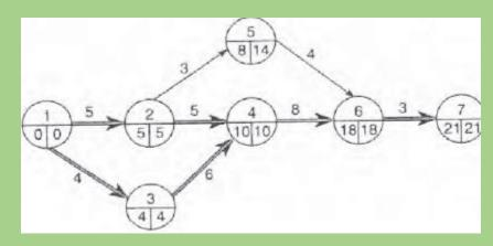
New Network Diagram is shown above. It is having Duration of 21 Days and the associated Total Cost is given as TC = Normal Direct Cost + Indirect Cost (for 21 Days @ ₹ 100 per Day) + Cost of Crashing Activity 1-2 by 1 Day = 4700 + 21 × 100 + 1 × 200 = ₹ 7000
