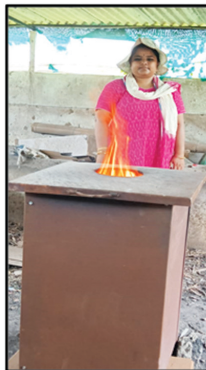
Image 1: Biochar production in TLUD
