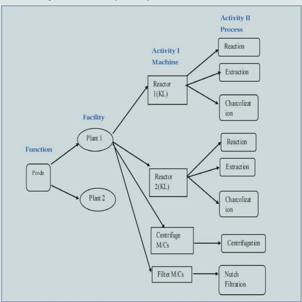
Note: Since multiple operations can be carried out on Reactors the lowest activity level is a combination of Machine & Process
