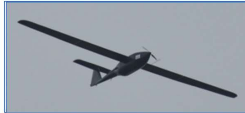
Hybrid Tiger leverages NRL's Ion Tiger long-endurance hydrogen fuel cell demonstrator: 26hr endurance on gaseous hydrogen, 2008 48hr endurance on liquid hydrogen, 2010
