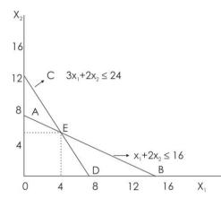
The optimal solution is at E (4,6) where P =₹48 but at D (8,0) also P = ₹48. Hence it means that all the points at E D boundary line, has got optimum solutions. Therefore the objective function is parallel to second constraint.
