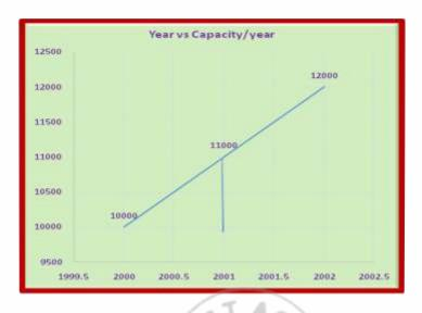
Area of the Right angle triangle shown with hypotenuse (10000-11000) is  $\frac{1}{2} * 1 * 1000 = 500$  is the no of units produced in the first year. Area of the Right angle triangle shown with hypotenuse (10000-12000) is  $\frac{1}{2} * 2 * 2000 = 2000$  is the no of units produced in the first two years. From this if we subtract 1<sup>st</sup> year production then production in 2<sup>nd</sup> year will come out as 2000-500 = 1500 units.
